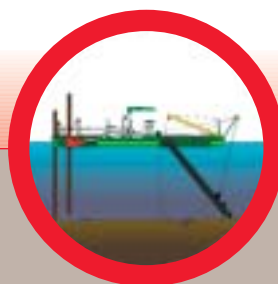
Step 2: Lowering of auxiliary spud
