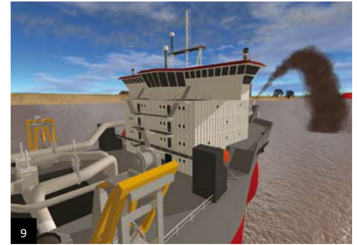
9 Rainbowing – the colour of the 'rainbow' reflects the mixture density that is actually discharged
